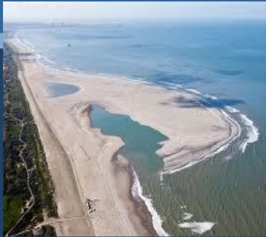
'Sand motor' beach replenishment, Ter Heijde, Netherlands
