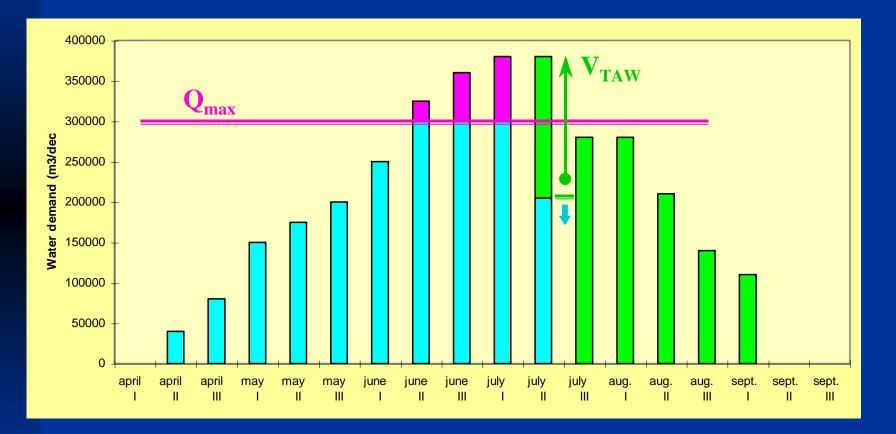
Constraints: Max. Flow Rate and Total Available Water
